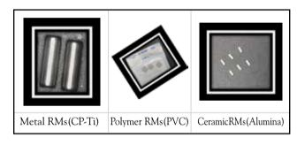
Figure 52. Reference materials for metal, polymer and ceramic classes
