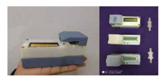
Figure 40. Chitra blood flow meter and flow tube
