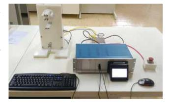
Figure 49. Terminal connection endurance test
