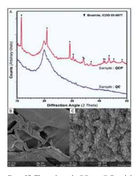
Figure 27. The results on the QC-nanoCaP graded membrane: A) The precipitated phase identified in XRD, B) the result of the in vitro bioactivity test wherein apatitic layer gets deposited from SBF, C) a magnified image of a region in B showing the thick layer formation.
