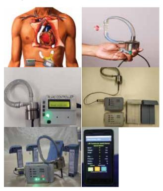
Figure 38. Chitra paracorporeal Left Ventricular Assist Device with controller, battery pack and charging unit
