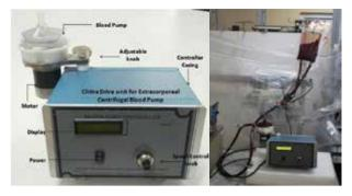
Figure 39. Extracorporeal blood pump, controller and drive unit
