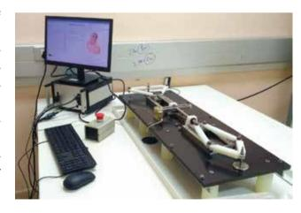
Figure 47. Lead body flexion testing
