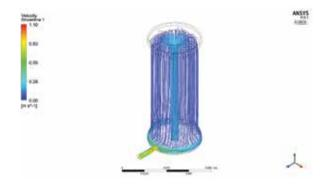
Figure 45. Computational fluid dynamics analysis of oxygenator - flow velocity streamlines
